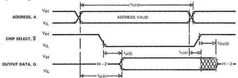
All timing reference points are 0.8 V and 2.0 V on inputs and 0.6 V and 2.2 V on outputs (90% points). Input rise and fall times equal 10 nanoseconds. †Write enable is high for a read cycle.
