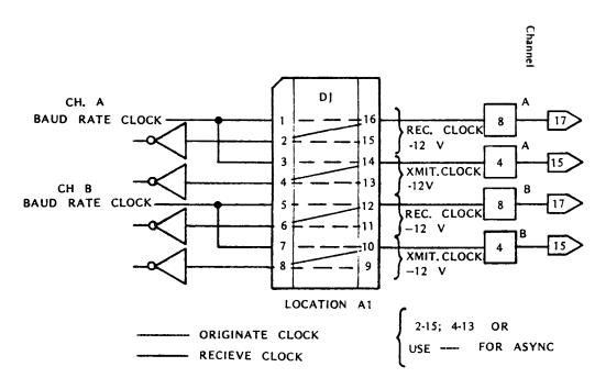
Program 8251 for x16 for asynchronous operation, x1 for synchronous.
