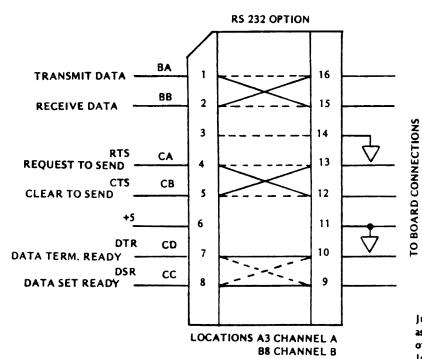
Jumpers shown for connection as terminal or computer end of an RS232 line.
