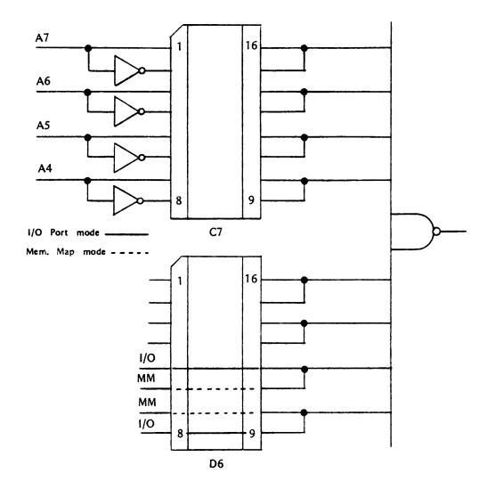
The board address is selected by jumpers or a DIP switch in locations C7 and D6. There are two cases for which this board may be jumpered: 1) to respond to input/output instructions and 2) to respond to memory access instructions. The case of input/output instructions will be treated first.
